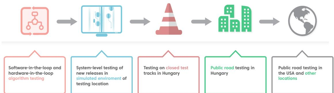
Figure 5: Almotive’s real-world testing happens as part of a 5-step process. Meetings of key decision makers conclude on when a certain build can move to the next step of the process based on all collected and available data.
