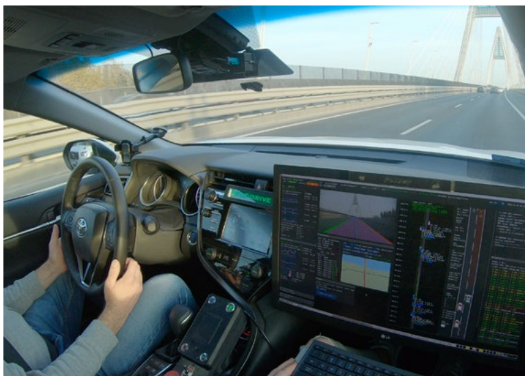
FIGURE 8. Currently, it is the responsibility of the Safety Driver and the operator to ensure that these conditions are met continuously during road testing. If any of them deteriorates, they deactivate the AD function.
